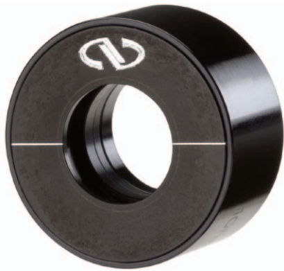
Figure 4. Newport 1/2 Wave-plate, model 10RP52-2 The line on the mount defines the azimuth of the wave-plate. If aligned at 45° relative to the input polarization direction, the output beam polarization is rotated by 90°.
